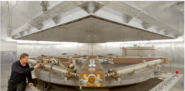
Ring laser „G“ in the underground lab
