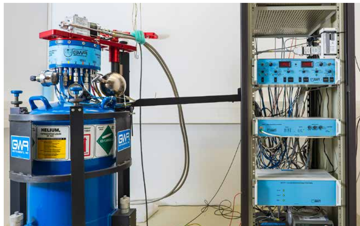
Supraleitendes Gravimeter GWR OSG Superconducting gravimeter GWR OSG
