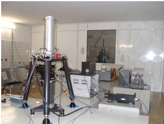
Figure 4. Micro-g gravimeter FG5 and superconducting gravimeter (background) at the ECGN core station Moxa (Germany)
